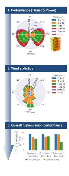
Wind propulsion can result in substantial savings in fuel consumption and exhaust gas emissions. Demonstration projects have shown that savings of 5% to 15% are immediately achievable in average wind conditions without really changing operations and ship design.
